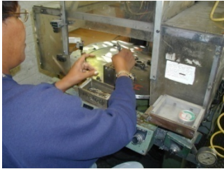
Magnet molding on meter shafts.
