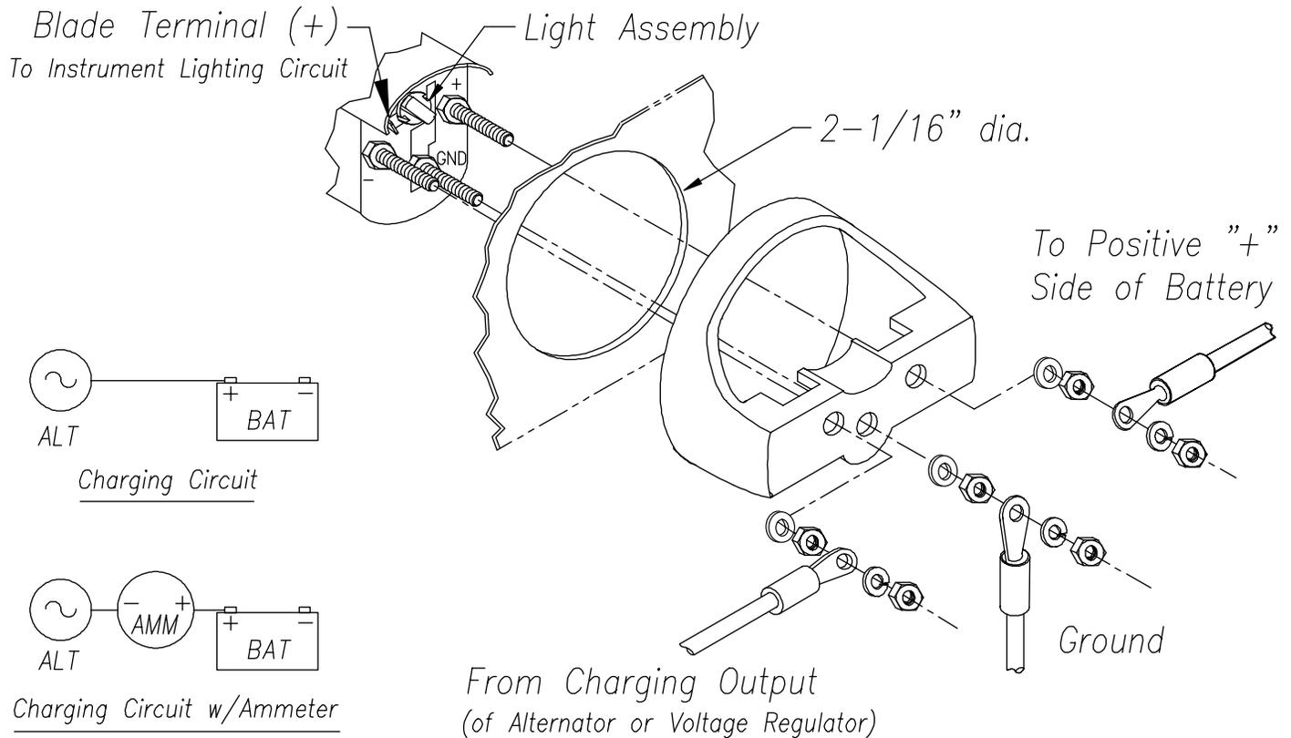
**CAUTION:** Disconnect the battery during installation. Tighten nuts on backclamp only slightly more than you can tighten with your fingers. Six **inch-pounds** of torque is sufficient. Over tightening may result in damage to the instrument and may void your warranty.
