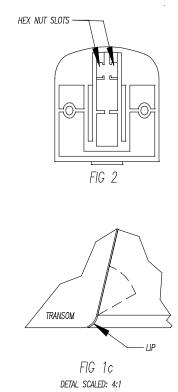
until the bottom of the paddle wheel support is parallel to the bottom of the boat with it's small "lip" hooked against the transom's bottom. (Refer to figure 1c). Tighten the two machine screws. Holding the sensor in the desired location, trace the outline of the mounting holes onto the transom. NOTE: It may be necessary in some applications to tilt the paddlewheel support deeper than parallel to increase high-speed sensitivity.
