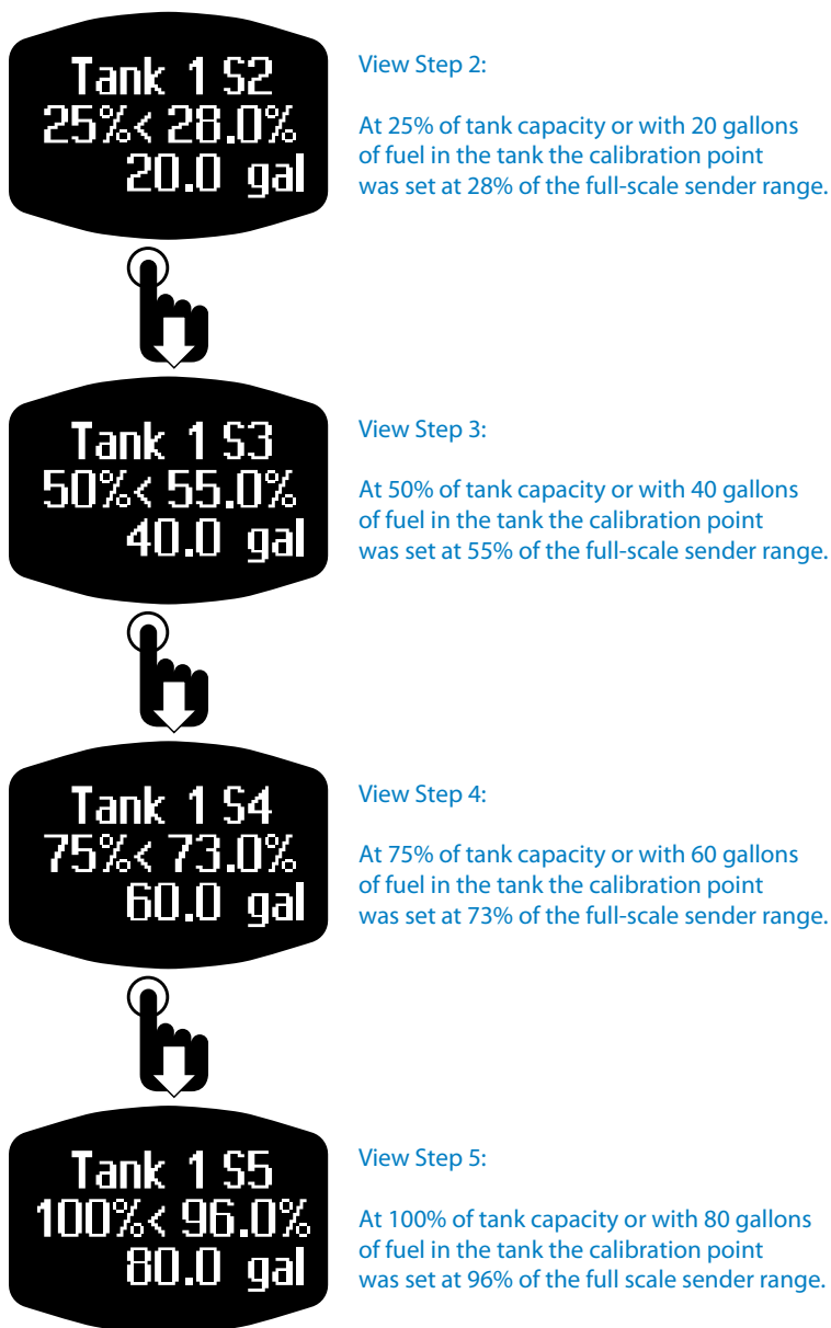
Figure 1-56: Viewing Fuel Tank Calibration Steps 2 thru 5
