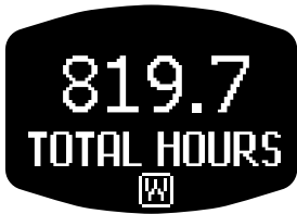
Figure 1-11: Quick View Main Screen with Warning “W” Icon
