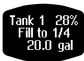
Figure 1-53: Setting Tank Calibration Points for 25-100%
