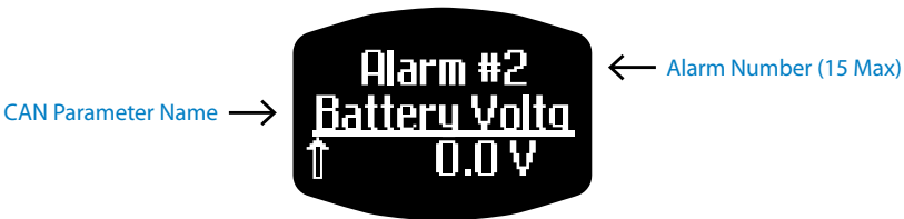
Figure 1-29: CAN Parameter Alarm Configuration Screen Detail
